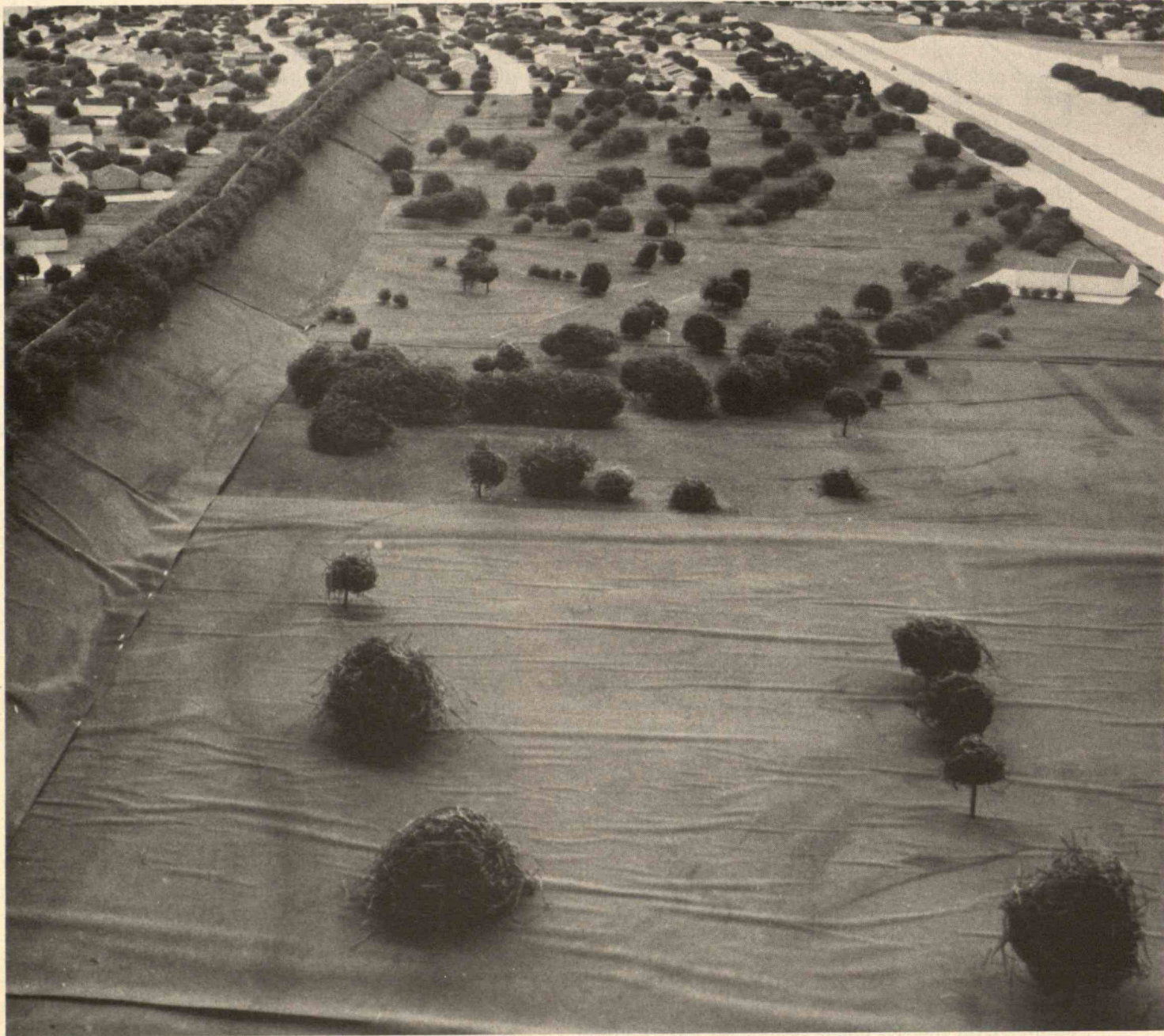
A 1:80 scale model of a Los Angeles Airport runway and the surrounding neighborhood allowed the author to study various methods of shielding communities from airplane noise.
