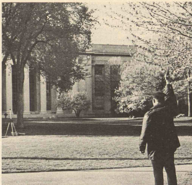
A campus patrolman shoots off a pistol in an M.I.T. courtyard to measure noise propagation for comparison with model data.
