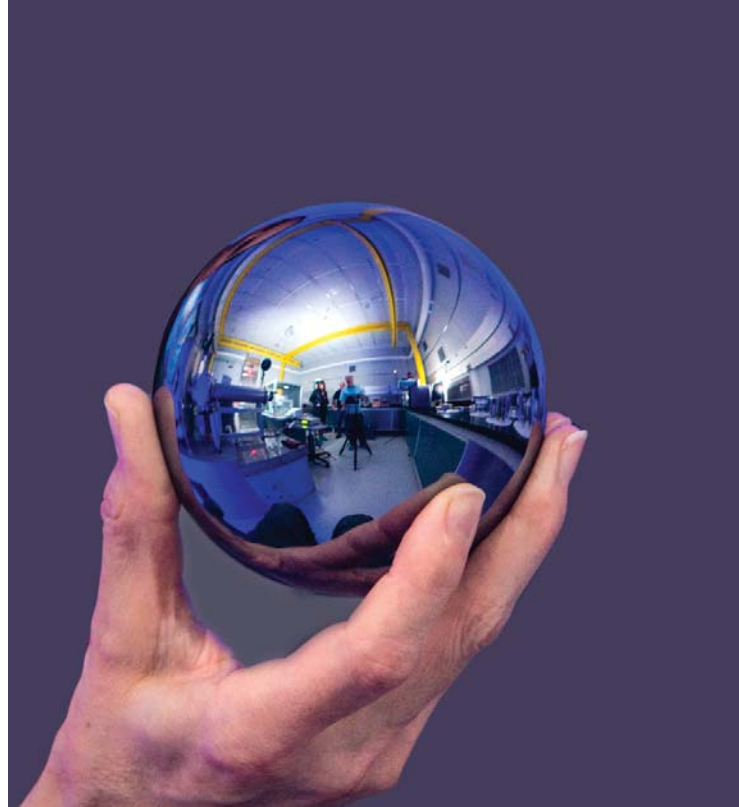
FIGURE 2. A SILICON SPHERE like the ones used by the International Avogadro Coordination. The IAC measured the diameters and lattice constants of the nearly perfect spheres to count the atoms and convert from the mass of a silicon atom to the mass of the silicon sphere. (Courtesy of NIST.)
